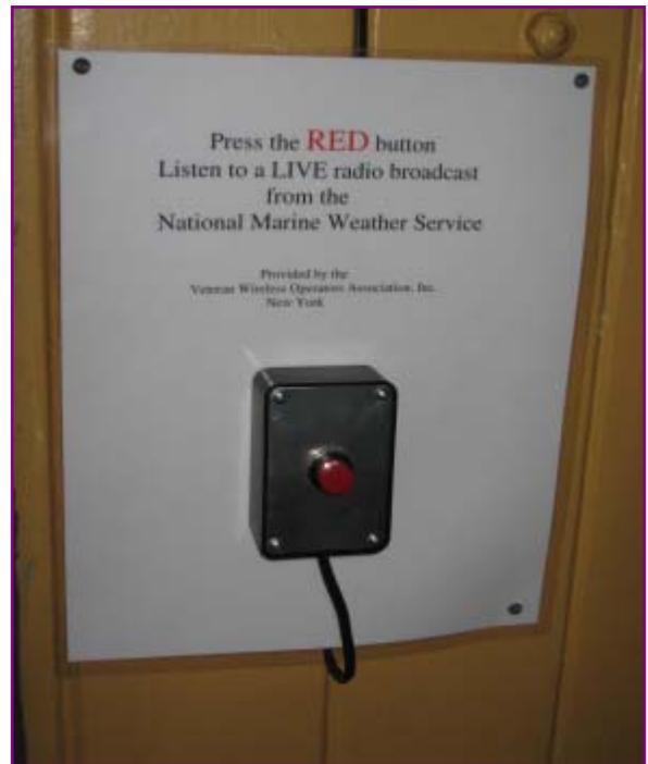
The RED button activates a marine weather radio for NOAA continuous broadcasts about the New York area. A speaker is mounted above the radio room door. The equipment is pre-tuned and doesn't require any manual operation. As long as AC power is on in the radio room, it's good to go.
