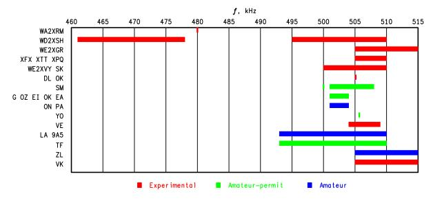
as shown in Figure 2. Three other US experimental licenses are also operating near 500 kHz.
