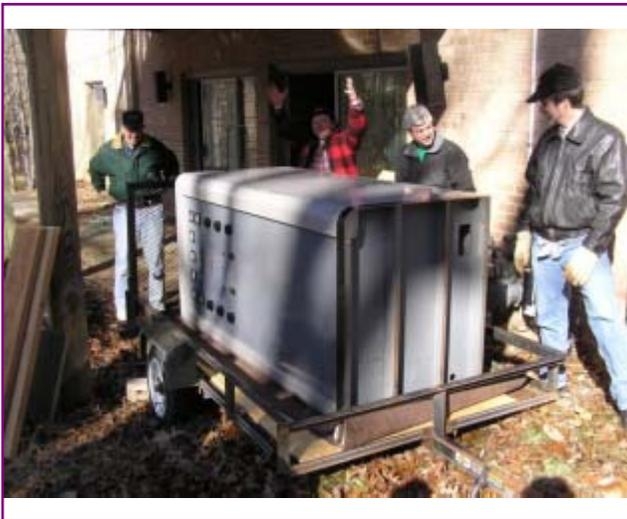
PHOTO 2: The BC-250GY transmitter removed from KOBRA's shack and loaded onto a small trailer, ready for transport up a grassy slope using manpower and a block & tackle secured to a suitable tree.
